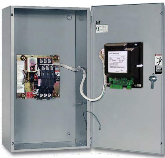
SERIES 300 Power Transfer Switch rated 200 amps
